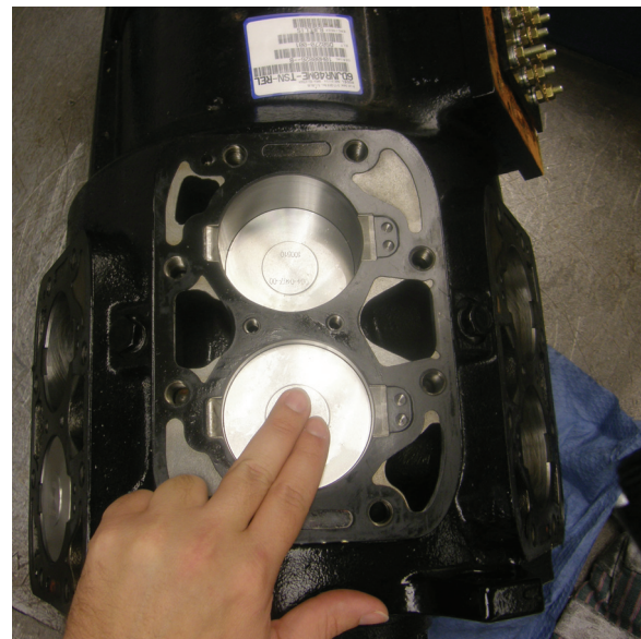
Figure 3 – Check that the pistons travel up and down freely by pressing down on each of the cylinders.
