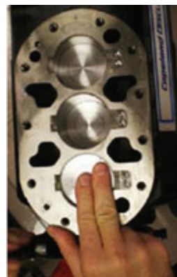
Figure 3 - Check that the pistons travel up and down freely by pressing down on each of the cylinders.
