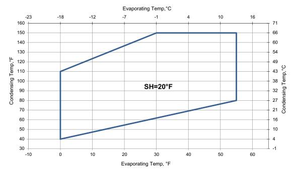
Figure 1B – ZS\*KAE Application Envelope for R-22 (Medium/High Temp)
