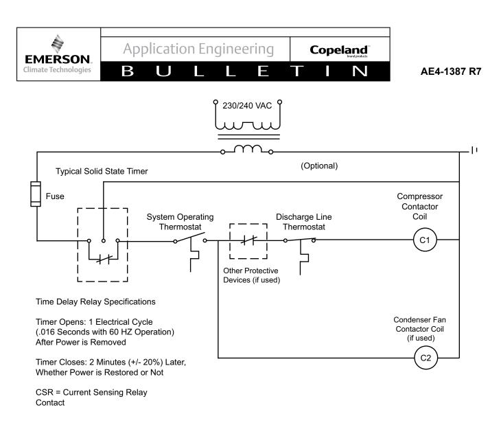
Figure 5 Scroll Wiring Schematic
