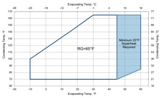
Figure 1C – ZS\*KAE Application Envelope for R-134A (Medium/High Temp)
