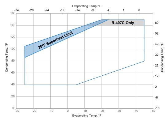
Figure 1D - ZS\*KAE Application Envelope for R-407A/407C/R-448A/R-449A (Extended Medium Temp)
