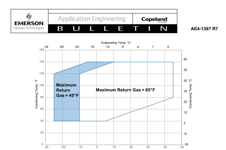
Evaporating Temp, °F Figure 1A – ZS\*KAE Application Envelope for R-404A/R-507 (Extended Medium Temp)
