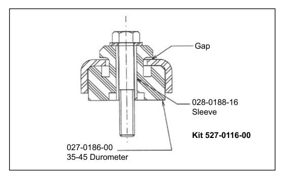
Figure 2B ZS21KAE to ZS33KAE Refrigeration Scroll 63 Frame Condensing Unit Mounting
